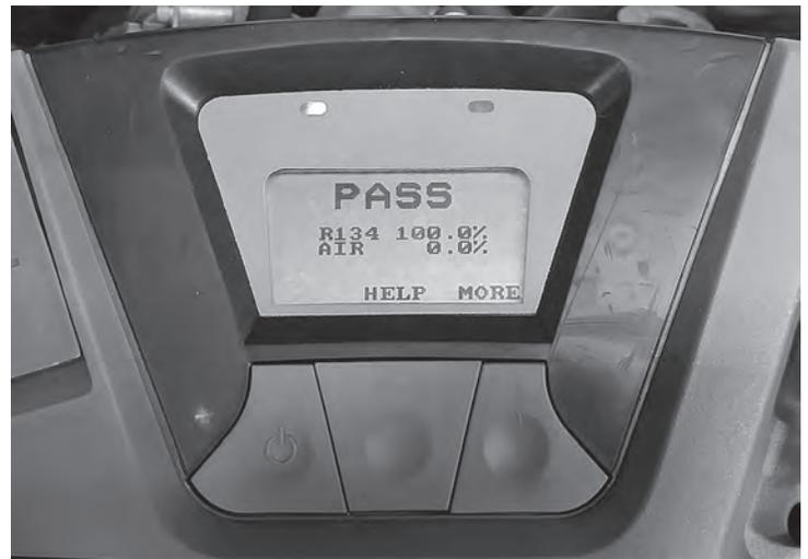
**An electronic refrigerant identifier is an essential tool to guard against refrigerant cross-contamination.**
