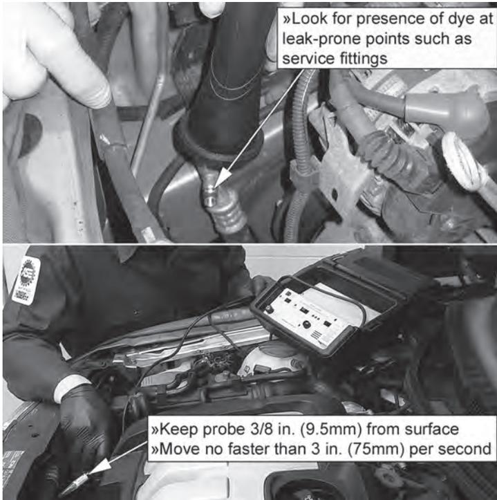
The procedures for using leak detection dyes (top) are covered by SAE standard J2298. Similarly, SAE standard J1628 covers the procedures for using electronic leak detectors (bottom).
