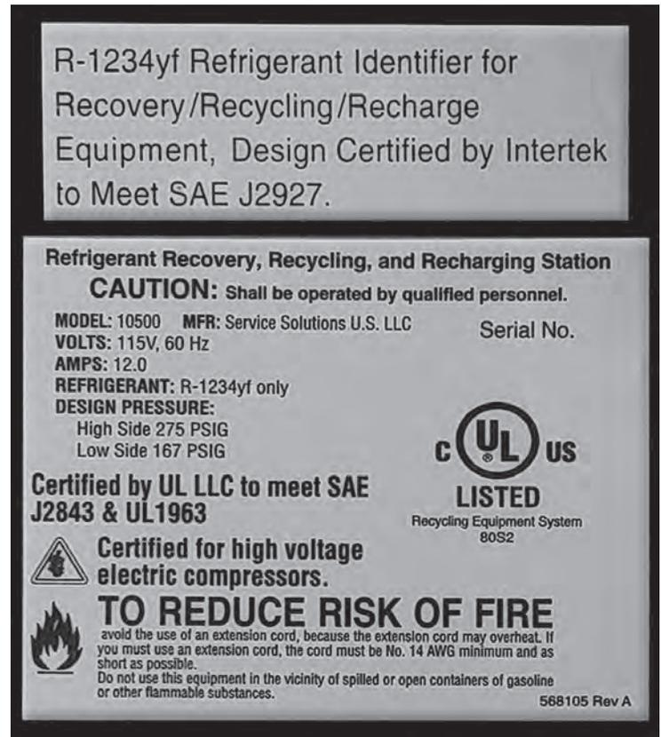
Refrigerant recovery and recycling equipment for R-1234yf must meet SAE standard J2843. This machine's label demonstrates compliance not only with J2843, but also SAE J2927 which applies to the machine's internal refrigerant identifier.
