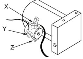
6. The liftgate motor above will not run when the circuit is energized. Battery voltage is present at terminals X and Y. To diagnose the problem, a jumper cable is installed across terminals X and Z.
