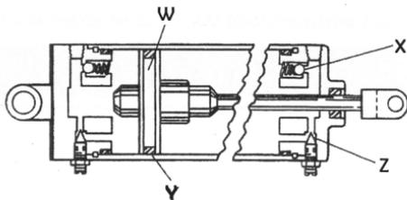
5. In the illustration shown, which of these is the piston seal?
