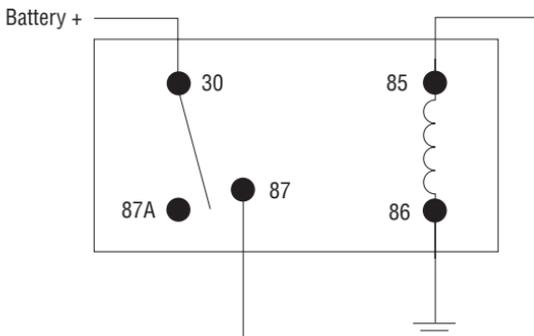
3. At which of the relay terminals shown would a technician check for a high current load when the relay is energized?
