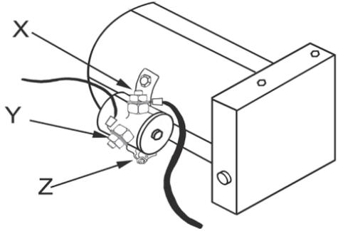
6. The liftgate motor shown in the illustration will not run when the circuit is energized. Battery voltage is present at terminals X and Y. To diagnose the problem, a jumper cable is installed across terminals X and Z. Technician A says that if the motor runs with the jumper cable installed, the motor solenoid could be the cause. Technician B says that if the motor does not run with the jumper cable installed, a bad ground could be the cause. Who is right?
